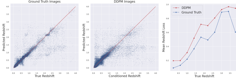
Figure 2: From left to right, the figure displays: 1) a scatter plot comparing predicted redshifts to true redshifts for ground truth images, 2) a similar scatter plot for DDPM-generated images, 3) a plot of true redshift versus mean redshift loss, highlighting the performance accuracy across the redshift range.
